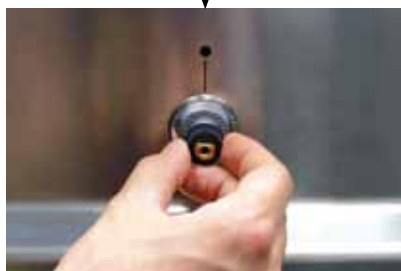
2 ... or push the adaptor onto the shaft
